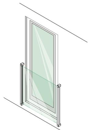
Installation onto the facade with vertical angular tube
